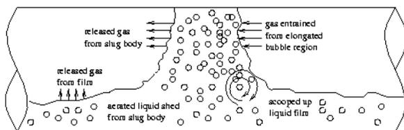
(a) Schematic of slug entrainment into a liquid slug
