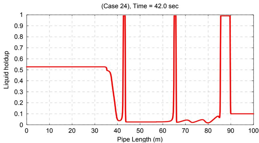
**Figure C1: Slug Flow Profile (Initiation, Growth & Propagation)**
