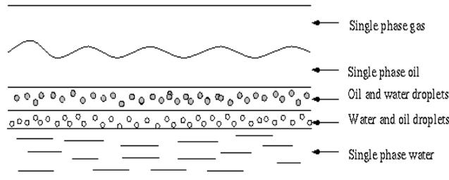
**Figure C6: Conceptual view of inter-phase mixing**
