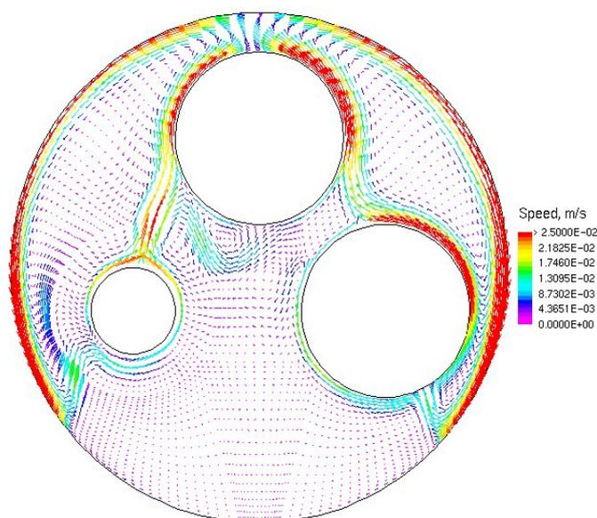
**Figure C9: Natural convection patterns in a multi-tube bundle**
