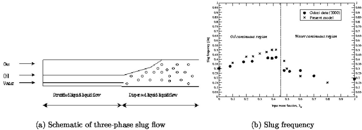
**Figure C8: Drift flux model for three-phase slug flow**
