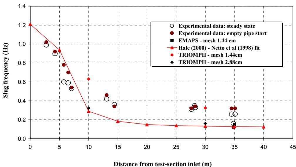
**Figure C5: Data for slug frequency obtained in the WASP facility**
