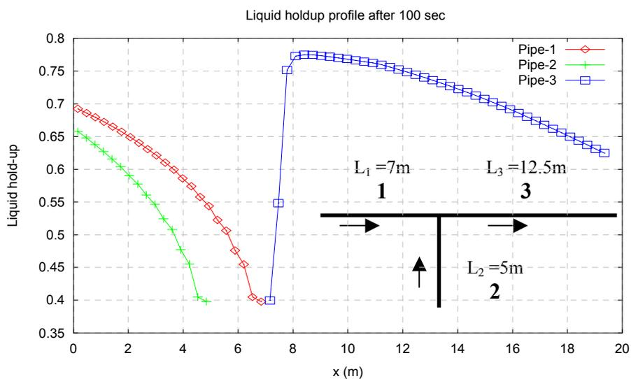
**Figure C2: Stratified Flow Profile in a Combining T-Junction**
